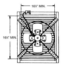
Figure 5 — Mounting to Rectangular Louvers
